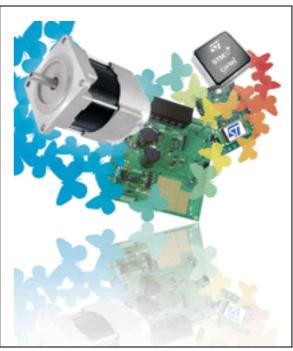
The kit comes ready-to-run with a PMSM motor or an AC induction motor (accessory). You can modify the demonstration application and develop your own motor control applications using the dedicated software libraries provided in the starter kit in conjunction with a third-party IDE and C compiler.
